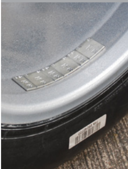
Tin alloy lead-free weight as developed for Bridgestone F1
