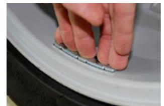
3. Grooves or a rough surface on the rim surface are also a problem. There is less surface for the adhesive to stick to, plus moisture can ingress under the tape from the ends. The Trax PROFESSIONAL tape is softer which allows a better fit to the inside of alloy rim surfaces which can sometimes be seen with “as cast” finishes or “orange peel” or machined grooves etc.
