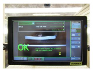
Two Cognex In-Sight 7050 cameras operate on each of the two lines and are required to inspect the correct orientation and size of the part, of which there are approximately 30 variants. Placed initially in a bowl feeder, the wheel weights are automatically positioned on a conveyor, which are then 'flipped' onto their side before being presented to the camera to check for the correct orientation and size.
